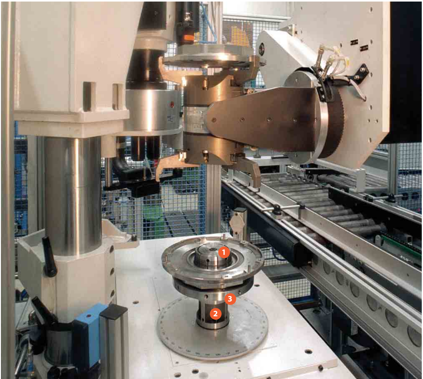
Vertical balancing machine integrated into an assembly line. Equipped with a RINGSPANN Collet Flange Mandrel ①, a Cylinder ② and an Axial Backstop ③.
