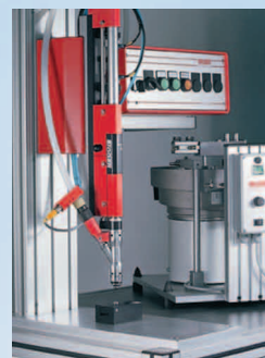
Screwdriver unit mounted on column
